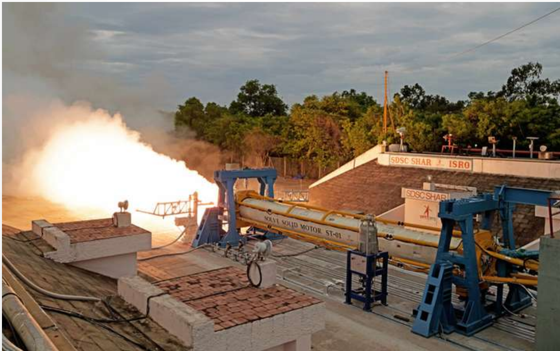
Photographic view during the Static Test of SOLVE-ST01
