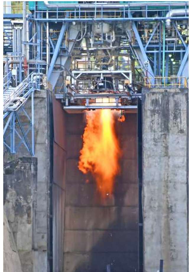
Photograph of E18 Engine Flight Acceptance Hot Test
